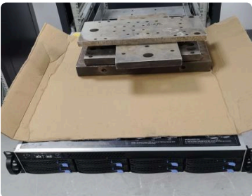
Load on the chassis, front view
